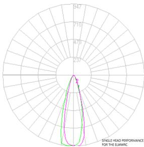
The ELWWRC is a wet location emergency light designed to illuminate the path of egress in environments where this fixture may be in contact with water. This includes two(2) adjustable heads rated at 300 lumens per head.
