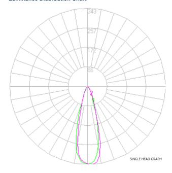
Initial Lumen Output: 200 lm Luminaire Type: Remote head Certification Standards: UL924, C22.2
