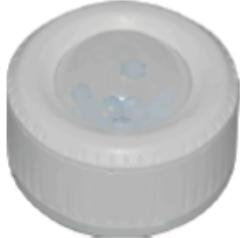
Z10-PIR mounts in an outdoor lighting fixture (street lighting, garden lighting, passageway lighting) and provides multi-level control based on motion and/or daylight contribution. It controls 0-10 VDC LED drivers or dimming ballasts, and is rated for wet and cold locations. All control parameters are adjustable via a wireless configuration tool capable of storing.
