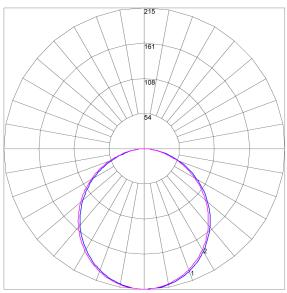
Maximum Candela = 215.002 Located At Horizontal Angle = 315, Vertical Angle = 1 # 1 - Vertical Plane Through Horizontal Angles (315 - 135) (Through Max. Cd.) # 2 - Vertical Plane Through Horizontal Angles (90 - 270)
